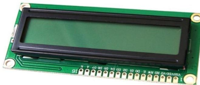
Figura 1. Pantalla LCD (chip.mecatronicum.com)
